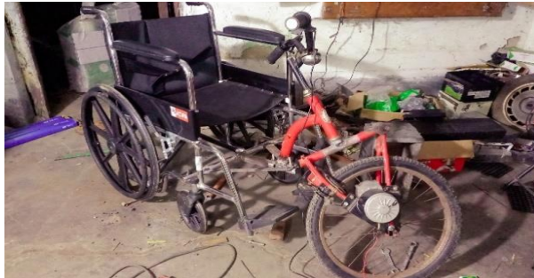
Figure 2: Prototype Model of an Affordable Electric Wheelchair
