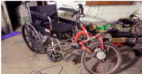
Figure 2: Prototype Model of an Affordable Electric Wheelchair
