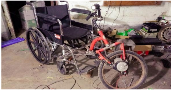
Figure 2: Prototype Model of an Affordable Electric Wheelchair
